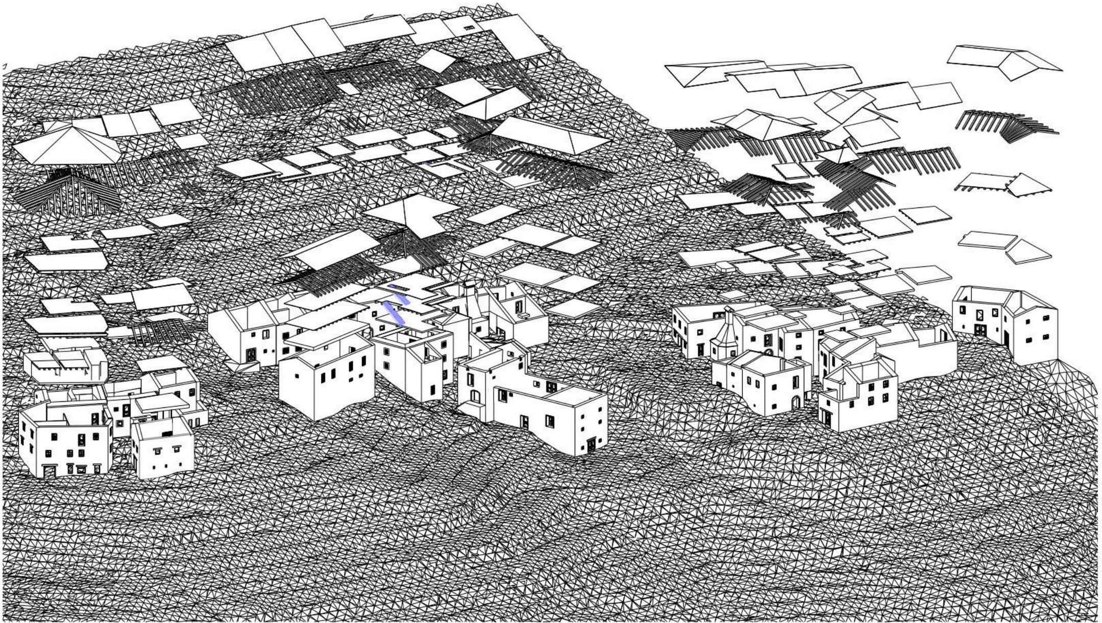
Exploded Axonometry of reconstructed buildings on site
