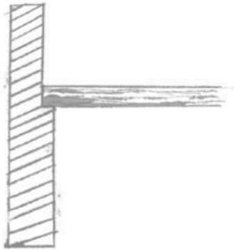
typical detail of wooden beams to walls connection
