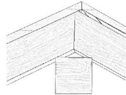
roof wooden beams to rafters connections
